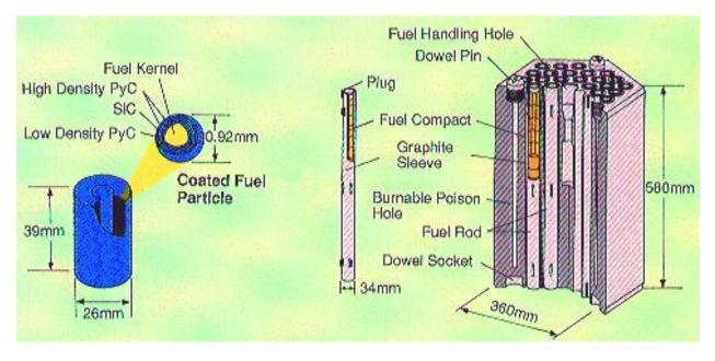
Figure 6. Prismatic graphite fuel assembly in the HTTR.
