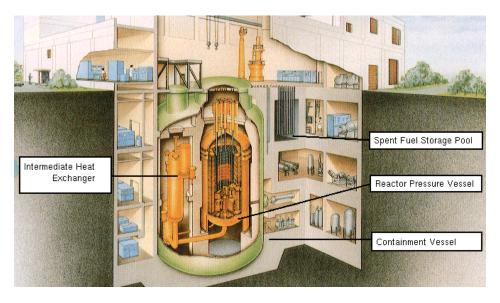
Figure 5. High Temperature Gas Cooler Reactor, HTTR, Japan.
