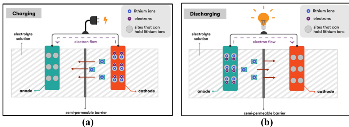
Figure 4: Diagrams showing the electronic and ionic transport processes that occur within a battery as it: (a) charges, and (b) discharges. 7
