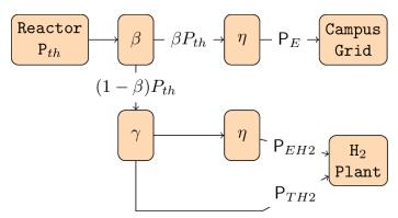
Figure 5. Diagram of a nuclear reactor coupled to a hydrogen plant [1].
