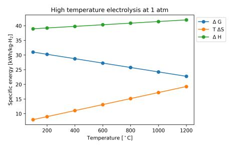
Figure 3. Energy required by electrolysis at atmospheric pressure [1].
