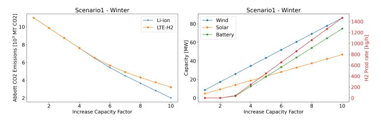
Figure 9. CO<sub>2</sub> emissions, wind, solar, and storage capacities for different increase capacity factors in the winter month.
