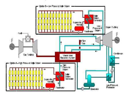
Figure 2. Integrated Solar Combined Cycle, ISCCS thermal system [2].
