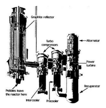
Figure 2. Diagram of the Pebble Bed Modular Reactor (PBMR).
