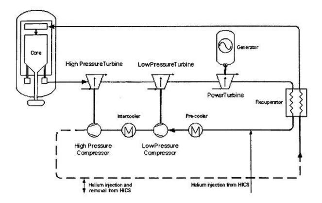
Figure 3. Flow Diagram of the Pebble Bed Modular Reactor (PBMR).
