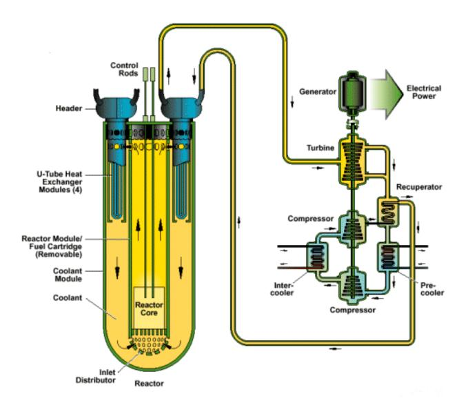
Figure 4. Lead Cooled Fast Reactor. Source: INL.
