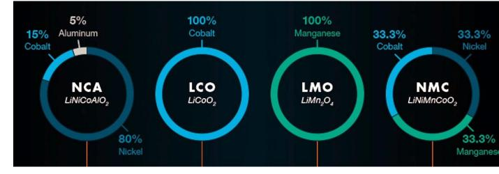
Figure 5, Types of Li ion batteries used by different car manufacturers. Li is the 25<sup>th</sup> element in abundance on earth. Aluminum, Nickel, Cobalt, and Manganese are also used. Electronics such as phones and laptops use Lithium Cobalt Oxide LCO chemistry batteries with a specific energy but a short lifespan as a 2 year life expectancy compared with 4 years for car batteries.
