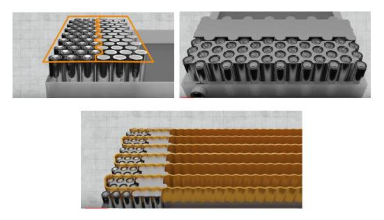
Figure 7. Battery pack bricks connected by a busbar in parallel. A cooling manifold asa ribbed interface that is a good heat conductor and good electrical insulator surrounds the cells and is cooled by a liquid water and glycol flow to a radiator.
