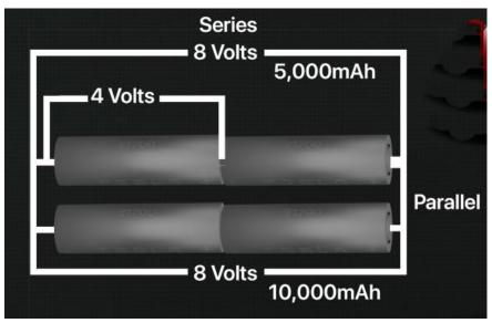
Figure 6. Tesla Cylindrical 2170 cells for battery pack is composed of 4416 lithium-ion battery cells in 16 modules wired in series for higher voltage or in parallel for higher capacity hence larger cruising range configurations.
